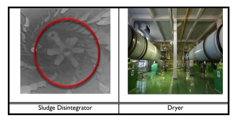
Sewage sludge consists of organic substances with high viscosity and high moisture content. Therefore, unless the particles are atomized in the initial phase of drying, a sticky zone with moisture content of 40 - 50% is formed as drying progresses, resulting in the formation of sewage sludge mass. Consequently, even if thermal energy is continuously supplied, only the surface of the sludge mass is dried leaving moisture inside. As a result, drying efficiency is lowered rapidly.
