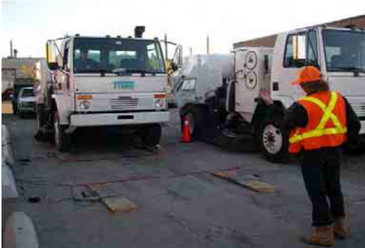
Figure 16: Portable Axle Weigh Scale
